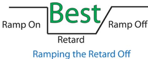
Ramp Off is used to control how quickly the timing is ramped back in after the slip condition is corrected. A Ramp Off setting of about 1/10<sup>th</sup> of a second is a good starting point; with a longer ramp in if more retard is used. If the amount of power reduced during a slip condition is too great, then a smaller retard may be required. If the tires recover from a slip condition and immediately slip again, then a longer RAMP Off may be desired.
