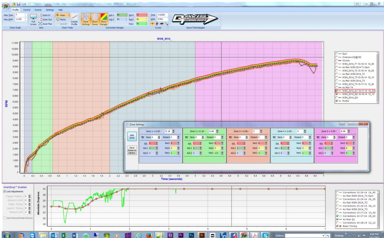
This is a screenshot of the Profiler software, showing the ‘ideal’ Driveshaft curve (the dotted line) and the correction ranges above and below it, and also the various zones (highlighted in colour).
