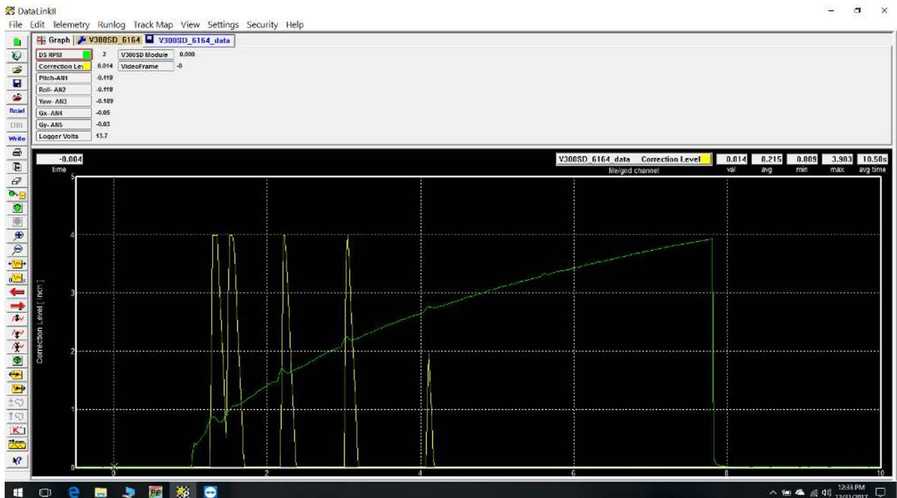
This image shows a Racepak data file of the Self learning traction control at work on a Pro Stock style car. The green line is driveshaft RPM, and the bumps in the curve show loss of traction (in this case on the gear shifts). The yellow line shows the corrections of the traction control system, the final correction being smaller in magnitude due to the loss of traction being less severe than the previous ones.
