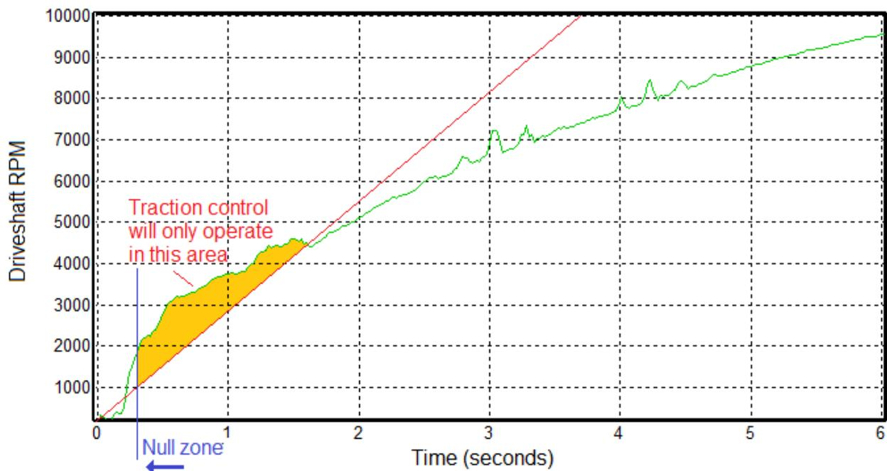
The diagram shows a null zone at the beginning of the graph where the rate of acceleration of the driveshaft is clearly greater than the predefined limit of acceleration. This zone is where the non self-learning system will not make any corrections until the driveshaft has reached the 'starting RPM'. This is necessary, as the driveshaft RPM is not linear, and thus the system must allow the car to get through this period of high driveshaft RPM acceleration before cutting the engine's power.
